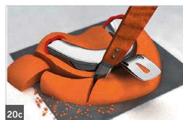
Fig. 20 c: Once the gypsum is cuttable, it can be trimmed into the first shape by using a knife.
