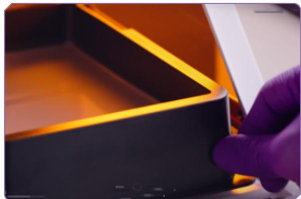
Always make sure that the windows inside the printer are free of dust and dirt.
