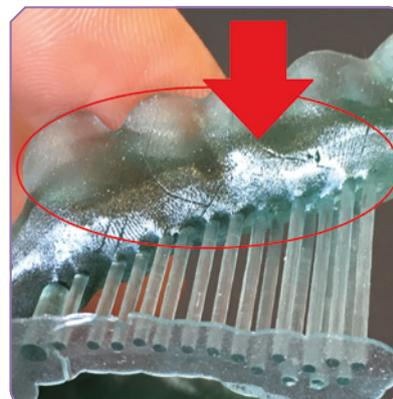
After cleaning, it is necessary to post-cure the printed pieces. Post-curing (post-exposure) is important, because it ensures the hardness and stability needed for dental applications and their biocompatibility.
