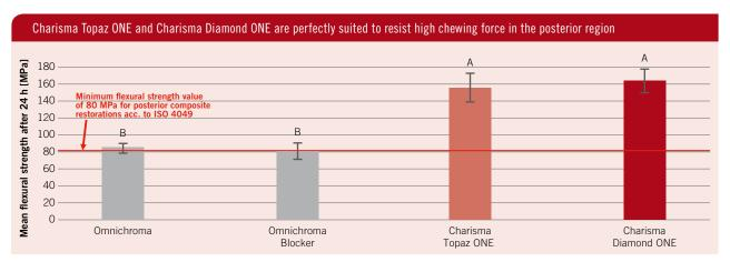
Mean flexural strength were for Omnichroma  $84.8 \pm 6.4$  MPa, for Omnichroma Blocker  $81 \pm 9.3$  MPa, for Charisma Diamond ONE  $164.2 \pm 14$  MPa and for Charisma Topaz ONE  $155.6 \pm 16.9$  MPa. Charisma Diamond ONE and Charisma Topaz ONE showed statistically significant higher flexural strength (p < 0.0001) than both Omnichroma shades. Same upper letters between materials indicate no statistically significant differences.
