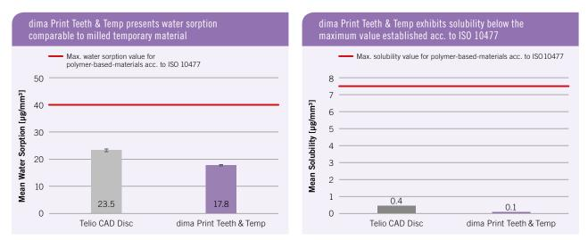
Water sorption and solubility were not measured for Telio CAD Block. The results of water sorption were statistically significantly different between the materials (LSD  $\alpha$ =0.05). All results of water sorption and solubility fulfil the ISO 10477 requirements.
