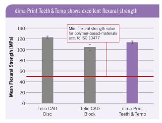
Mean flexural strength (standard deviation) of Telio CAD Disc was 122.7(2.3) MPa, of dima Print Teeth & Temp was 113.8(2.3) MPa, and of Telio CAD Block was 103.5(5.8) MPa. The results were statistically significantly different between the materials (LSD  $\alpha$  = 0.05).
