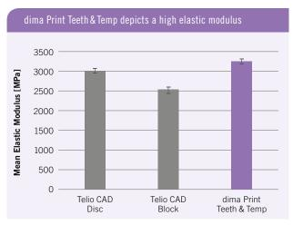
Mean elastic modulus (standard deviation) of dima Print Teeth & Temp was 3268(49)MPa, for Telio CAD Disc 3031(52) MPa and for Telio CAD Block 2538(87)MPa. The results were statistically significantly different between the materials (LSD  $\alpha$  = 0.05). For elastic modulus no ISO requirement is stated.
