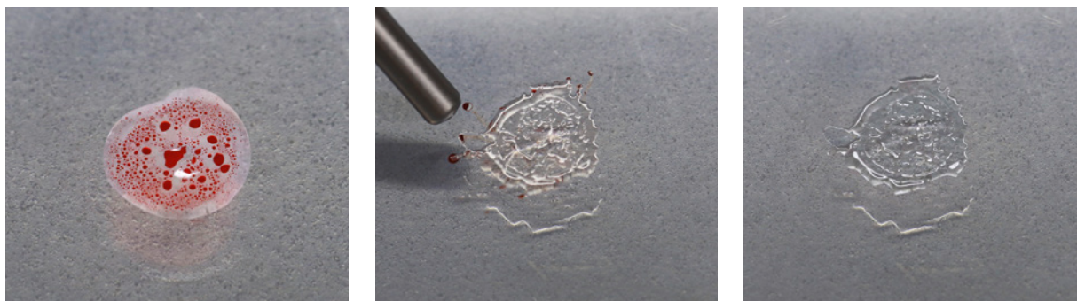
Fig. 9: Left: The aqueous phase was marked with a selectively soluble red dye, while the monomer phase is colourless. Phase separation (separation of the oily monomer portions and the aqueous portions) is visible. Centre: The volatile components such as acetone and water are removed from the film by evaporation. Right: A colourless film remains. This illustrates the effective expulsion of water from the adhesive layer.
