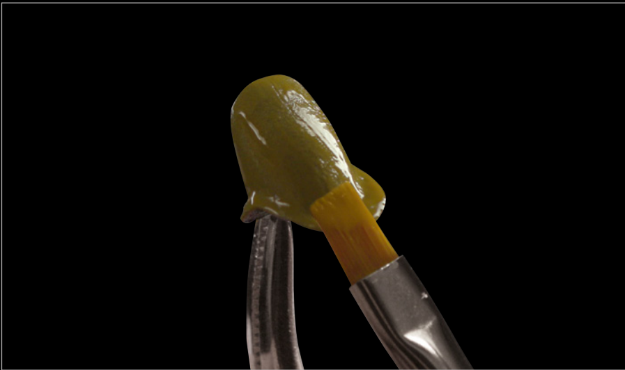
Fig. 9 NP-Primer applied very thinly (high brush pressure!) with paste opaquer brush.
